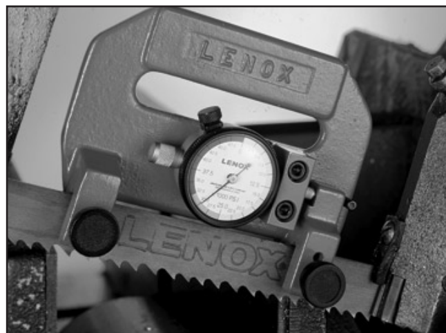
Figure 41. H5408 Blade Tensioning Gauge.
